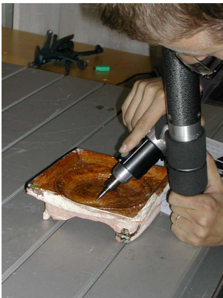
Picture 5. Esa Laine measuring details on a stove-tile with 3D coordinate measuring machine. Photo: Hannele Lehtonen.
