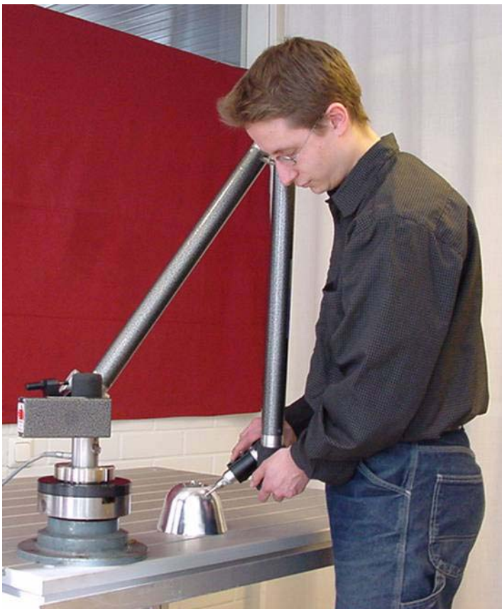
Picture 4. 3D Coordinate Measuring Machine (CMM) in the department of Mechanical Engineering of Turku Polytechnic School, with which the measurements of stove-tiles were made.
